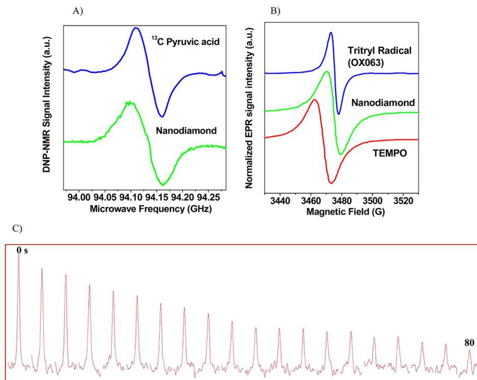
**Figure 2.** (A) Microwave sweep data at 1.4 K for  $^{13}\text{C}$ -pyruvic acid with 15 mM trityl radical (OX063) and nanodiamond samples. (B) Room-temperature X-band EPR spectra of OX063, nanodiamond, and TEMPO, over a sweep width of 100 G. Data were normalized to their peak values. (C) Representative dynamic array (horizontal) of  $^{13}\text{C}$  MRS of hyperpolarized nanodiamond after the dissolution process. A  $T_R = 4$  s was employed for this scan.
