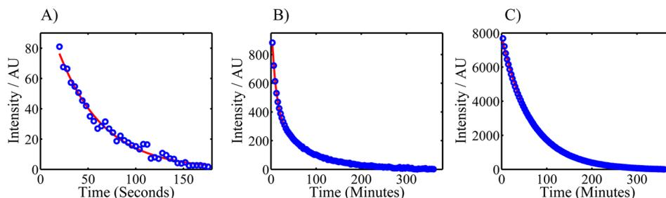
**Figure 3.** (A) Decay of the hyperpolarized  $^{13}\text{C}$  MRS signal intensity of nanodiamond at room temperature (the theoretical fit estimates  $T_1 \approx 55 \pm 3$  s). (B,C) The solid-state  $T_1$  measurement data at 1.4 K for nanodiamond and  $^{13}\text{C}$ -pyruvic acid, respectively.
