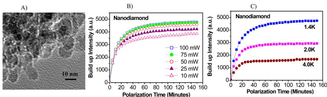
**Figure 1.** (A) Transmission electron micrograph (TEM) of the diamond nanoparticles dispersed in acetone. (B,C) The solid-state polarization buildup curve with polarizing time for different microwave powers at 1.4 K and for several temperatures at 100 mW of power, respectively.
